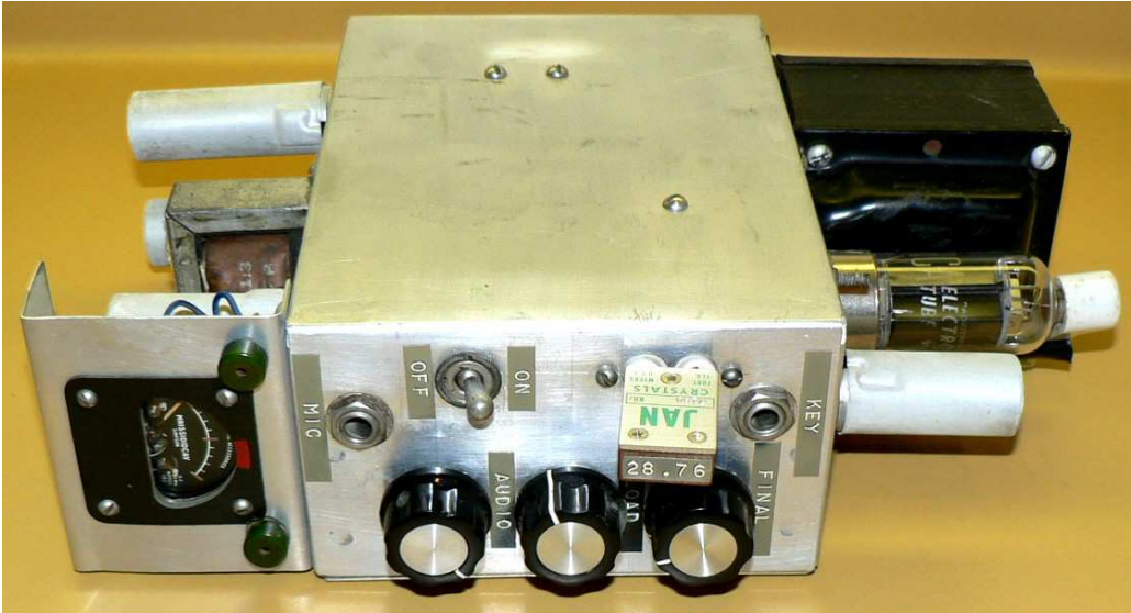
Ten-meter AM transmitter built by Quent Cassen and me for use in his parents' car.
