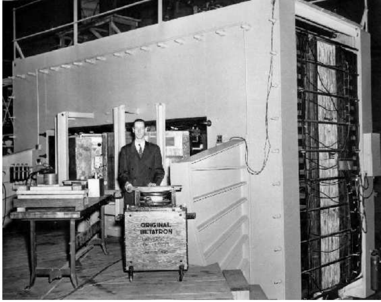
Don Kerst in front of the 400-ton, 300-MeV betatron in about 1950 at the University of Illinois and behind the original 200-pound, 2.3-MeV betatron, completed in 1940 and now on display at the Smithsonian Institution in Washington, DC.
