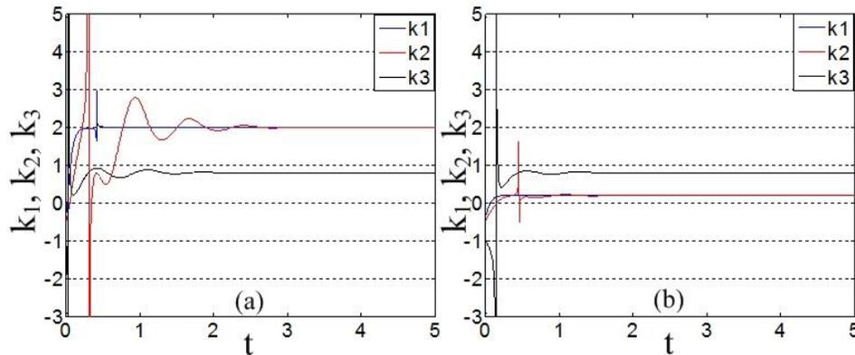
Fig.5. Behavior of the drive and response systems for same-phase projective synchronization (a)  $k_1 = k_2 = 2$ ,  $k_3 = 4/5$  (b)  $k_1 = k_2 = 1/5$ ,  $k_3 = 4/5$ .
