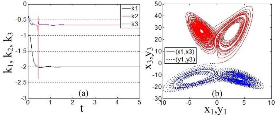
Fig. 4. Behavior of the drive and response systems with initial conditions (0.1, 0.1, 0.1) and (-0.3, -0.2, -0.1), respectively (a) anti-phase projective synchronization (b) projection onto the  $(x_1-x_3)$  (the solid line) and  $(y_1-y_3)$  (the dash line) plane
