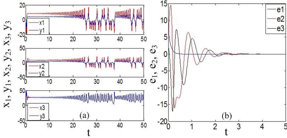
Fig.2. The time evolution of (a) signals (red line for drive system and blue line for response system) and (b) the error vectors with  $m = 1$ ,  $n = 4$ .
