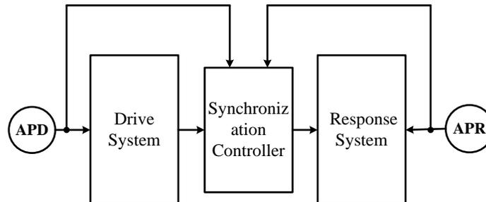
Fig.1. The projective synchronization system model
